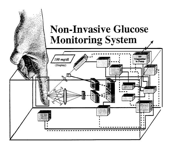
Figure 1. Non-invasive glucose monitoring system. This finger represents only one of several different sites for analyzing concentrations of blood glucose and other constituents.
