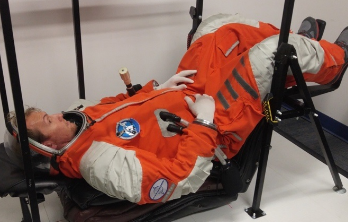
Figure 3. Final Frontier Design’s demonstrator spacesuit in spacecraft cabin mockup during 2016 Project PoSSUM.
