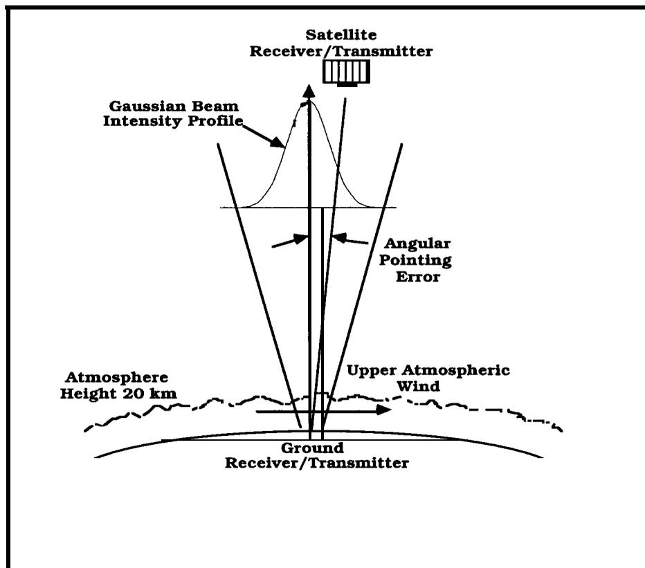
Fig. 1. Schematic of the up-link propagation channel, illustrating the Gaussian-beam profile of the mean intensity at the satellite and the relative pointing error. The satellite will orbit at 350 Km
