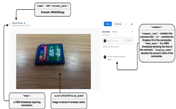
Figure 6. A demonstration of an individual file preview showing comment information and file metadata.
