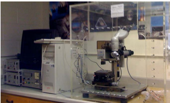
Figure 3. CSM Revetest Scratch tester with glovebox enclosure for humidity reduction
