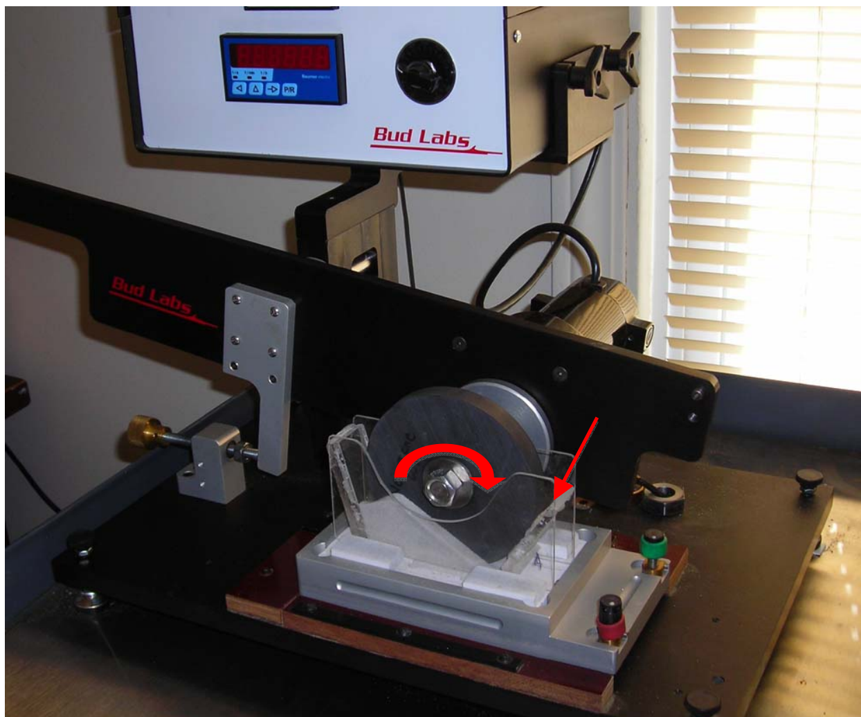
Figure 1.—Three-body abrasion tester (rotation direction indicated with curved arrow) with abrasive entry point on right side (indicated with straight arrow). The specimen sits at the bottom of the rotation wheel.
