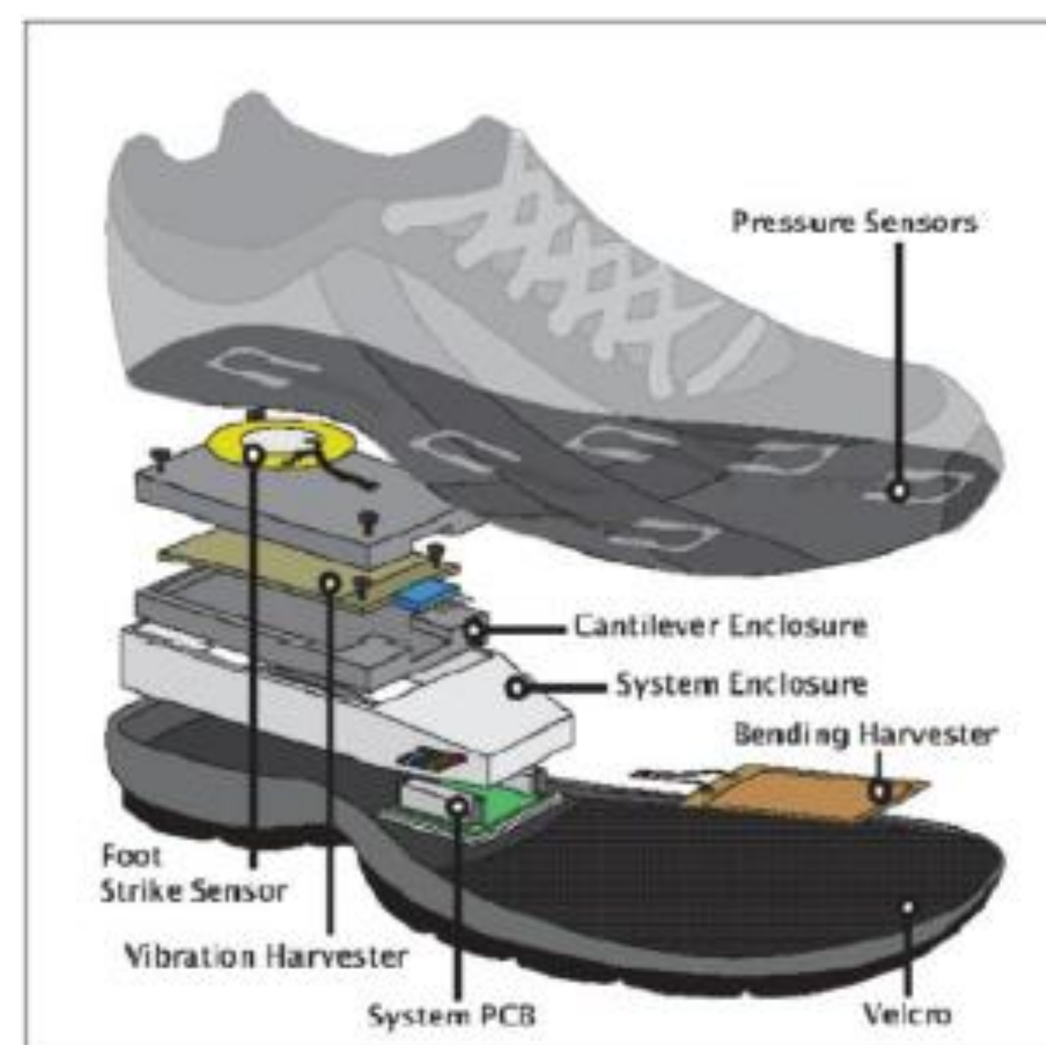
Figure 1 Basic composition of a smart shoe [1]
