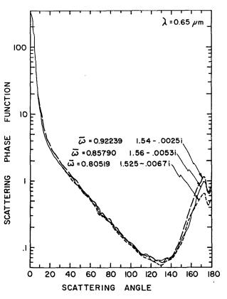
FIG. 3. Phase functions and single-scatter albedoes computed from three refractive indices.
