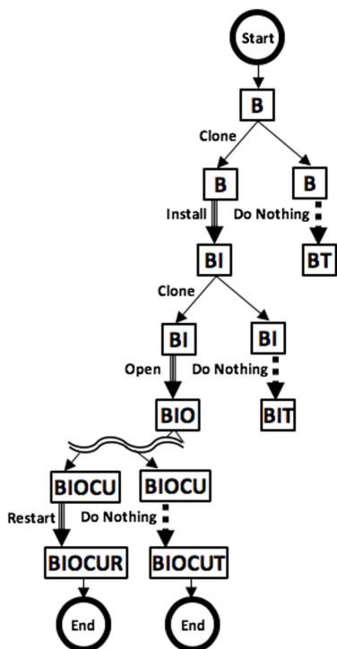
Figure 2. Overview of the VM buildup procedure for "application-run" and "do- nothing" branches with respect to catalog creation.
