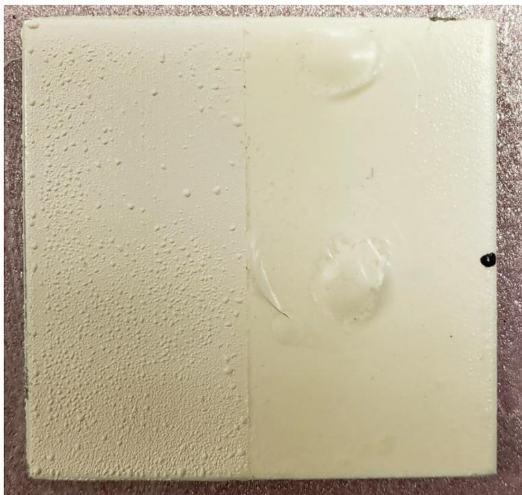
*Figure 4.11* Coupon D texture: 156 min total exposure
