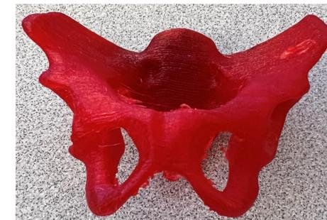
The printer the pelvis was printed on is the FlashForge Creator Max 2, however the team has recently concluded the purchase of an Ultimaker S5 printer to further expand their 3D printing capabilities. The pelvis was printed using SainSmart 95A Red TPU Filament.
