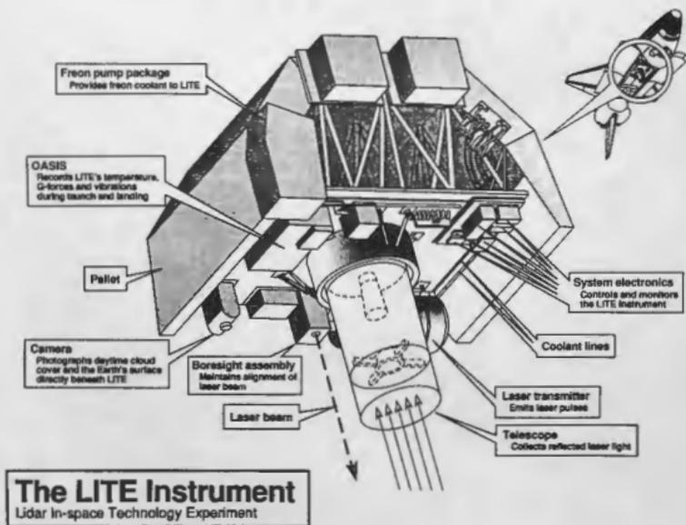
Figure 1. A depiction of the LITE instrument and its configuration aboard Space Shuttle Discovery
