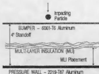
Figure 3. Typical Whipple Shield
