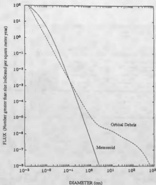
Figure 1. Comparison of Meteoroid and Orbital Debris Flux
