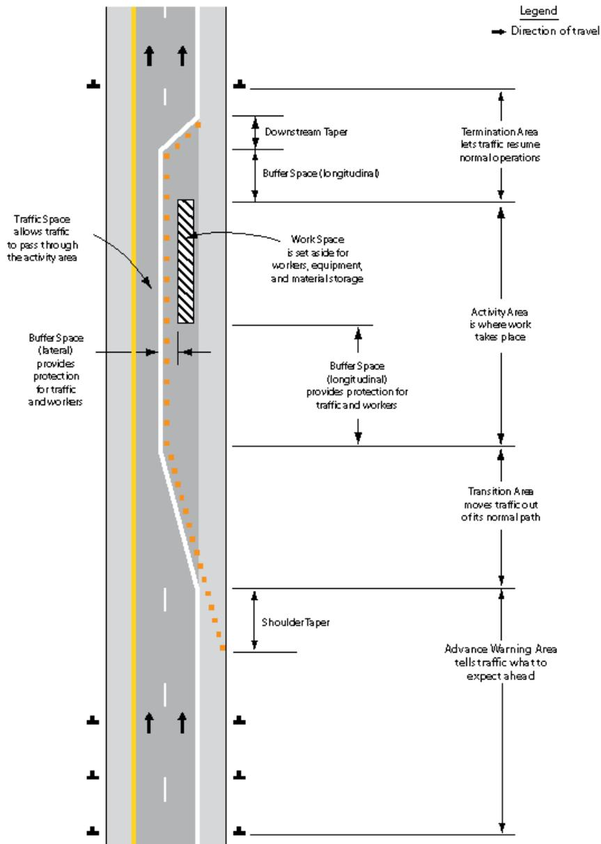
Figure 4 - Diagram of cone taper for incident management response (U.S. DOT and FHWA, 2021)
