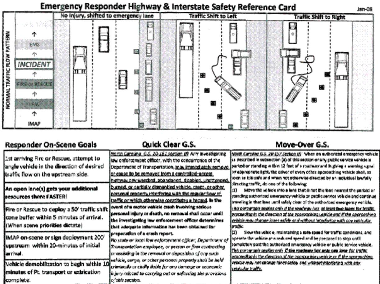
Figure 5 - North Carolina DOT Emergency Responder and Interstate Safety Card Reference (U.S. DOT and FHWA, 2021)
