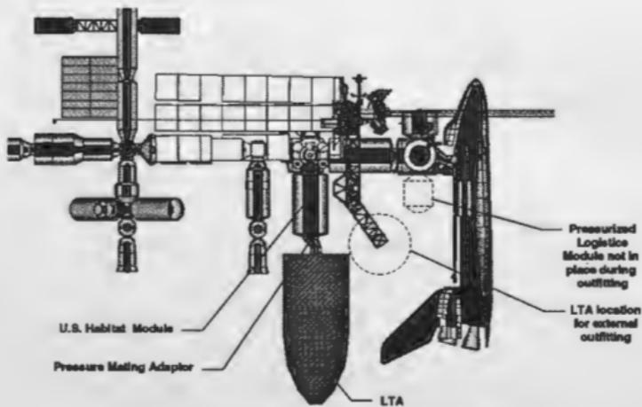
Figure 5. LTA Docked for Internal Outfitting
