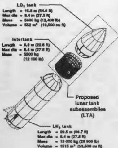
Figure 1. NSTS External Tank Subassemblies
