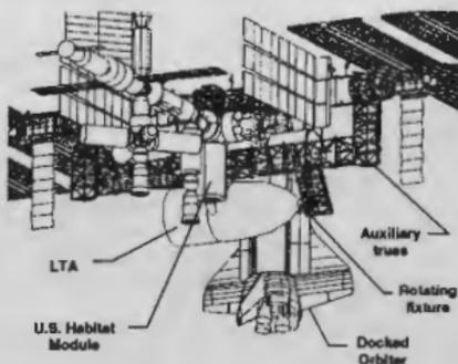
Figure 4. LTA Docked at ISSA Auxiliary Truss
