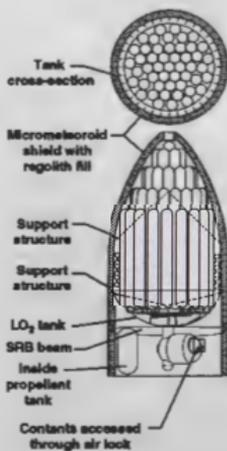
Figure 6. LTA Configuration for Cryogenic Storage of Helium-3
