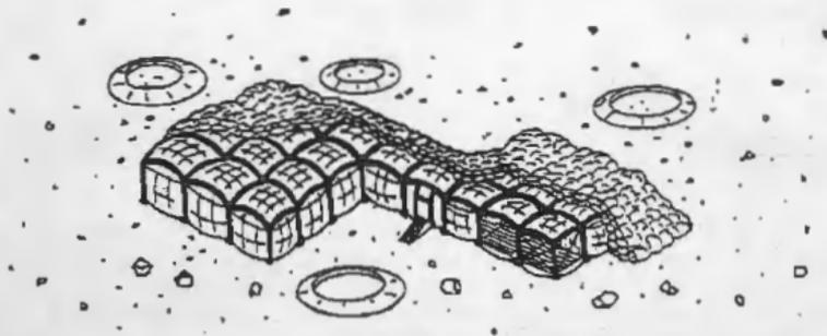
Fig. 1 An overall view of a lunar inflatable structure consisting of two clusters of identical modules.
