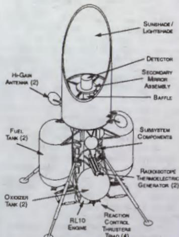
Fig. 4. LTT Reference Design Concept.
