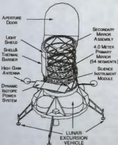
Fig. 3. LCTE Reference Design Concept.
