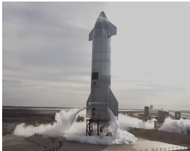
Figure 2.3: Starship SN15 Body [12]. Note the wide non-symmetrical cross-section of the vehicle which makes it difficult to control a gravity flip turn in the upper atmosphere
