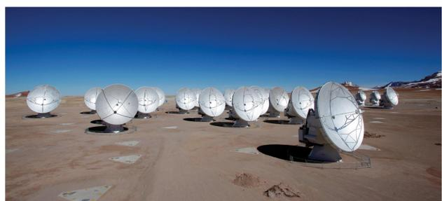
**Figure 2:** The Atacama Large Millimeter/Submillimeter Array (ALMA) telescope, (located in Chile) has 50 antennas and can be arranged in many configurations. The telescope operates in the wavelength range between 0.32mm to 3.6mm. Credits: ALMA (ESO/NAOJ/NRAO).
