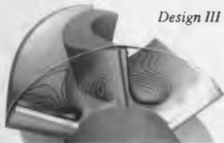
Figure 4 : Axial velocity contours at the exit plane of various LVAD impeller design
