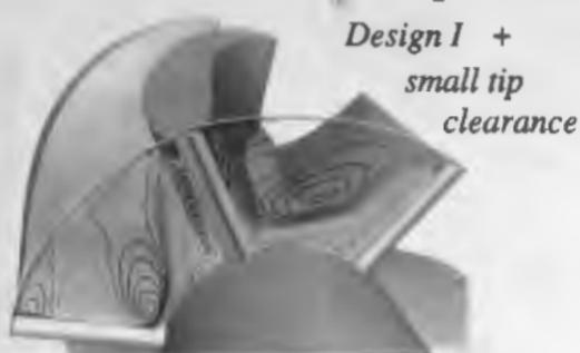
*Axial Velocity Contours at Impeller Exit*
