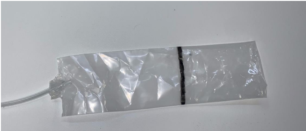
Figure 3: Fluidization Example - Half Eversion
