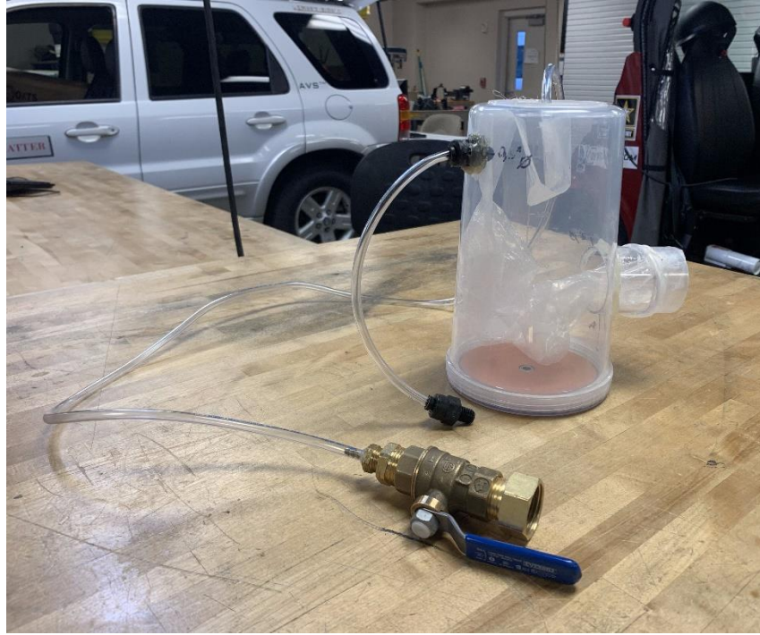
Figure 5: Design of Air System with Water Fluidization
