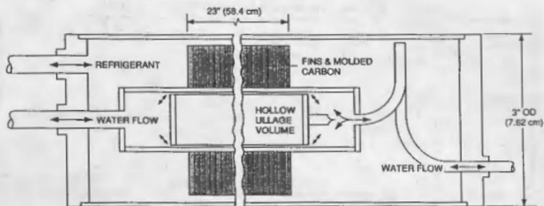
Figure 3. Sorption Compressor Assembly Cross-Section
