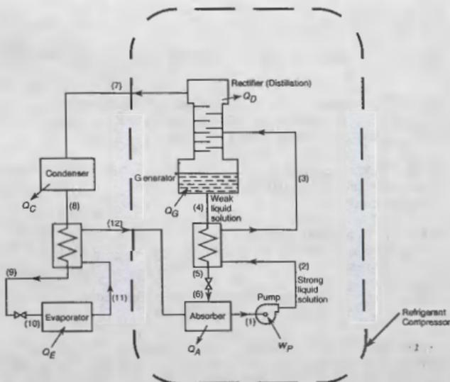
Figure 4. Common Liquid Absorption Refrigeration System
