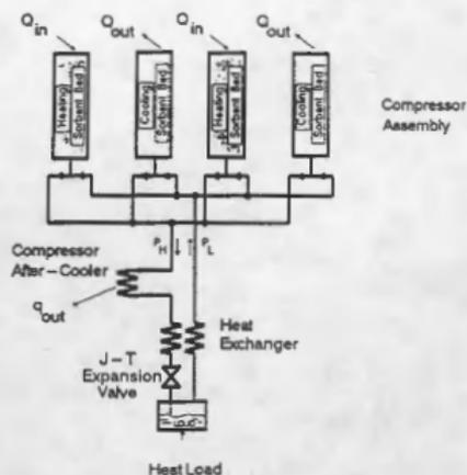
Figure 1. Basic Sorption Refrigeration Concept
