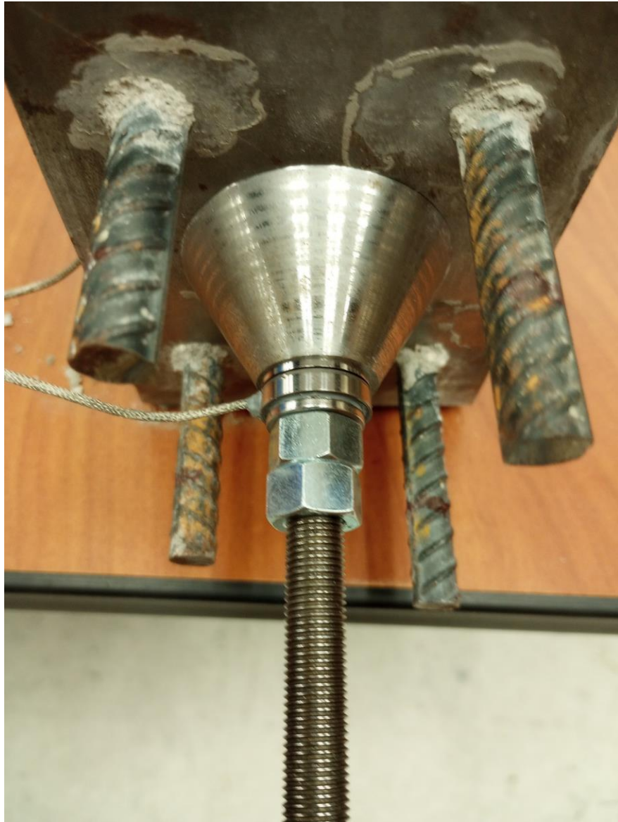
Figure 14 Picture showing load cell used for post-tensioning measurements on scale-beam
