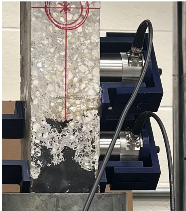
Figure 8 Example of the external mount for the non-hardening bonding methods with 50kHz transducers
