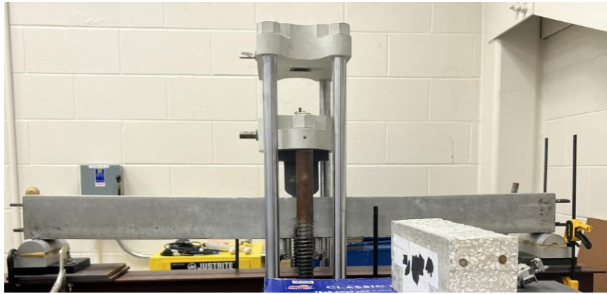
Figure 15 Picture showing the 3-point load testing setup for the PT-scale-beam
