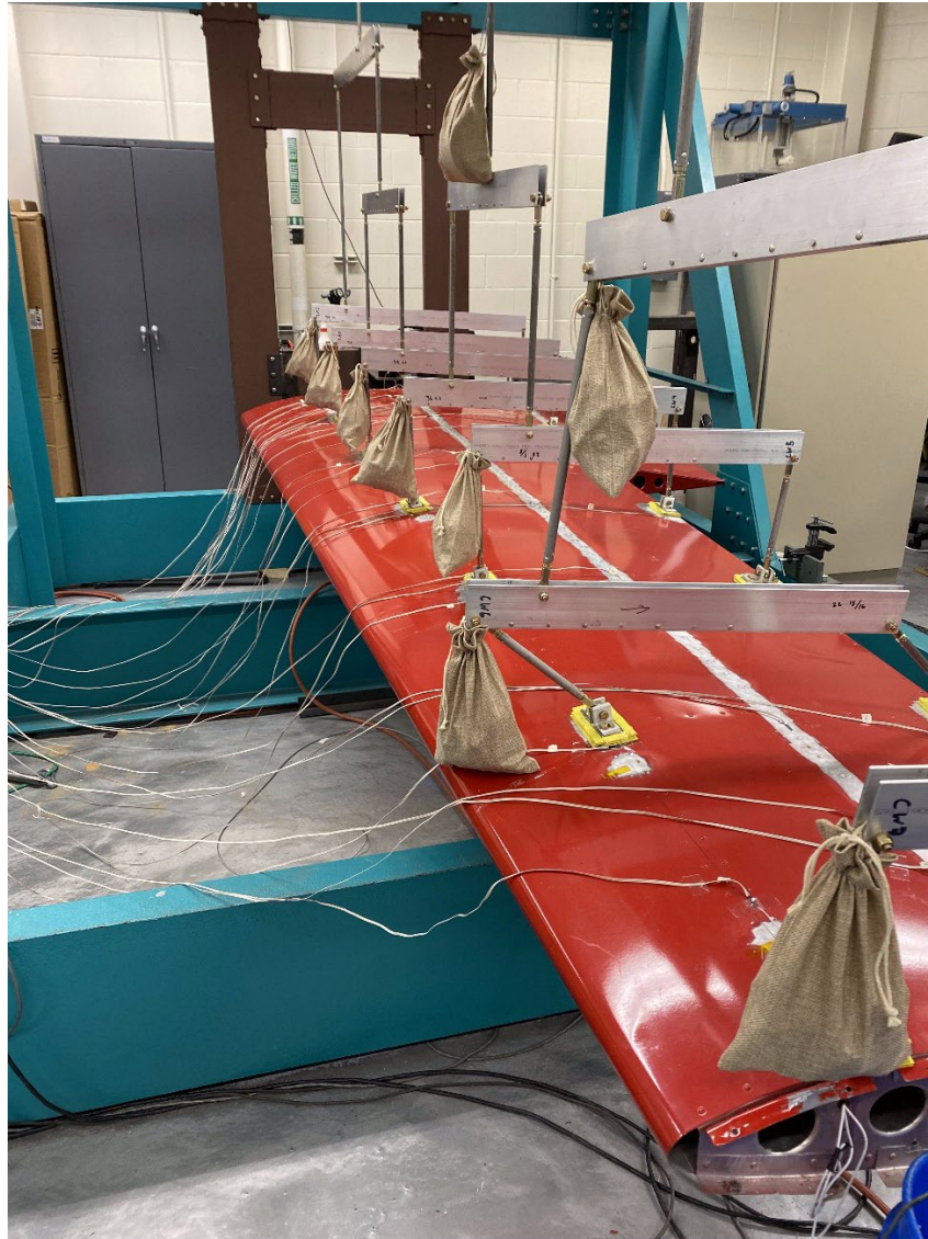
Figure 5.1 Light Sport Aircraft Wing with Counterweights.
