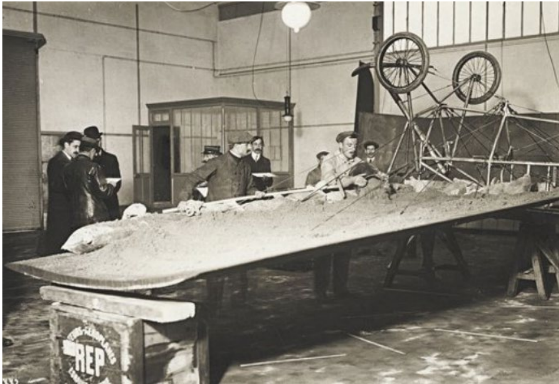
Figure 1.1 Static Testing of a Monoplane Wing using Sandbags in 1911 [1].
