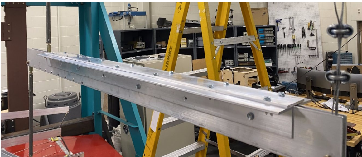
Figure 5.2 Channel Section Adhered to SWB2.
