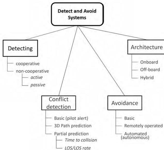
**Cooperative Technologies** – Cooperative sensor technology is used to receive signals of intent from other aircraft equipped with compatible avionics and to determine their position. Cooperative sensors usually have larger range than non-cooperative technology and are more reliable.
