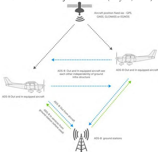
New advancements in commercial ADS-B have allowed it to be integrated into sUAS with minimal size/weight/power impacts. Use case examples for using transceivers for DAA can found elsewhere (Harvey & O’Young, 2015; Mitchel et al., 2020). Due to its limitations
