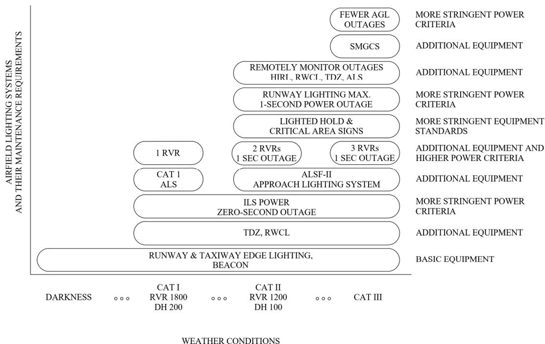
*Note:* This figure summarizes lighting system requirements included in AC 120-118 *Criteria for Approval/Authorization of All-Weather Operations (AWO) for Takeoff, Landing, and Rollout* and AC 120-578B *SMGCS*. The figure only shows three category levels, but several levels exist between these with modified criteria and requirements.
