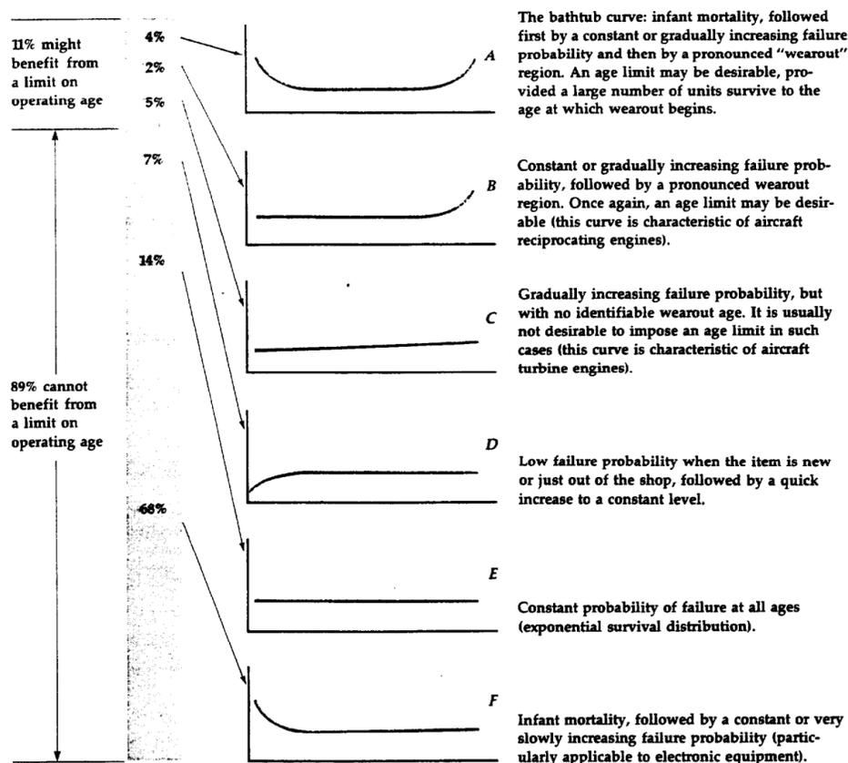
*Note.* The vertical axis represents the conditional probability of failure and, the horizontal axis represents operating age since manufacture, overhaul, or repair. The percentages show the percentage of items studied that fell into each of the basic patterns. Reprinted from *Reliability-Centered Maintenance* by Nowlan & Heap, 1978, Office of Assistant Secretary of Defense. In the public domain.
