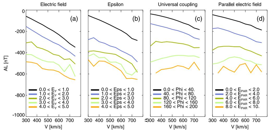
**Figure 1.** AL index as function of solar wind speed for five values of the driver function: (a) solar wind electric field  $E_Y$  in units of mV/m, (b) the  $\epsilon$  parameter in units of  $10^{11}$  W, (c) the universal coupling function  $d\Phi_{MP}/dt = (V^2 B_T)^{2/3} \sin^{8/3}(\frac{\theta}{2})$  in units of  $((m/s)^2 T)^{2/3}$ , and (d) the parallel electric field along the large-scale X line  $E_{PAR}$  in units of mV/m.
