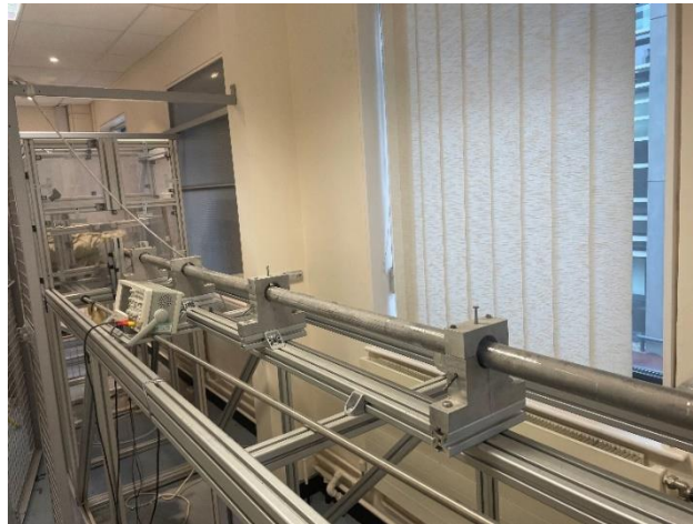
Gas Gun Chamber with an Oscilloscope and Impact Area
