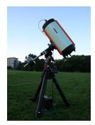
**Figure 1.** OSCOM telescope system for small satellite and debris photometry deployed in Needham, MA, USA. Used with permission from Gasdia et al. [14] © 2016 AMOS Conference.
