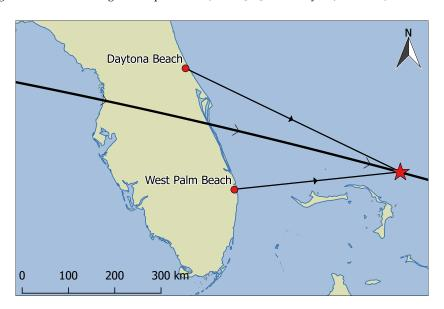
**Figure 9.** Geometry and ground track of the simultaneous observation of ASTRO-H Object A from Daytona Beach and West Palm Beach, FL on 7 May 2016. Object A at 09:31:05 UTC is marked by the star.
