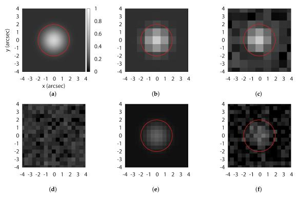
**Figure 2.** Effect of sampling a two-dimensional Gaussian of 2 arcsec FWHM (**a**) by image scales 1 arcsec/pix (**b**) and 0.5 arcsec/pix (**e**) and with source Poisson and Gaussian read noise (**c**,**f**). Sample detector read noise is shown in (**d**). Red circles represent 2 arcsec radii photometric apertures. All figures are at the same spatial and intensity scale.
