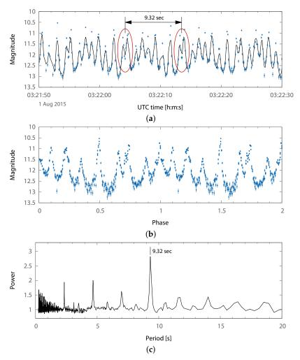
**Figure 7.** (a) light curve of the DICE-2 CubeSat (Spacetrack ID 37852) spinning at about 0.1 Hz. This observation occurred using the OSCOM system shown in Figure 1 from Needham, MA, USA using 125 ms integration time. The smoothing line is a five-point centered moving average. (b) phase diagram with five 9.32 s periods of the light curve from 03:21:45 UTC to 03:22:31 UTC overplotted. (c) Plavchan periodogram of the DICE-2 light curve showing a primary period of 9.32 s.
