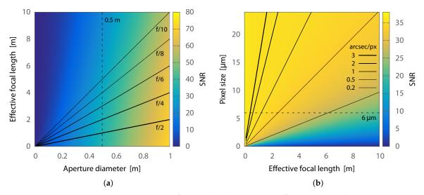
**Figure 4.** (a) aperture diameter, a proxy for area, has the strongest influence on signal-to-noise ratio (SNR) of an unresolved RSO. However, for a given aperture, there is also an improvement in SNR at shorter focal lengths. This plot assumes  $6 \, \mu m$  pixels; (b) oversampling an unresolved RSO spot reduces the photometric SNR by increasing the sky background and read noise for a constant 1 FWHM photometric aperture radius. This plot assumes a  $0.5 \, m$  aperture.
