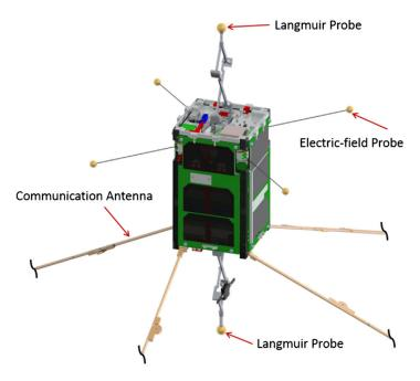
Figure 6. Diagram of the DICE CubeSat with deployables. Figure from Fish et al. [44].
