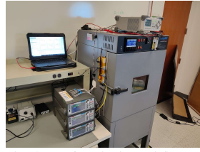
Figure 1: Image of the calibration setup in SAIL. Test Equity 115A shown on right. Left: Up to 3 Keithley 2450 sourcecurrents for simultaneous calibration.
