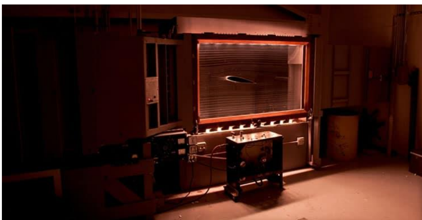
Shows 2-D flow visualization over an airfoil at the Lehman Wind Tunnel Laboratory
