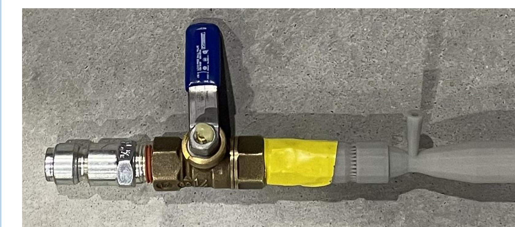
Test setup - duct & plumber's tape was used to secure the nozzle
