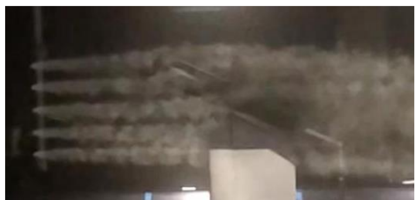
Shows the sheet of smoke at 10 fps. The turbulence is smoke is visible and the streaklines. The flow is a dispersed two-phase flow.
