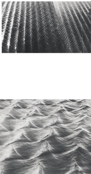
FIG. 2: (Top) Wave patterns in a basin showing two-dimensional subharmonic instabilities ( ak = 0.32 , f = 1.55 Hz). (Bottom) A typical three-dimensional spilling breakers in a basin. From Su et al. [14].
