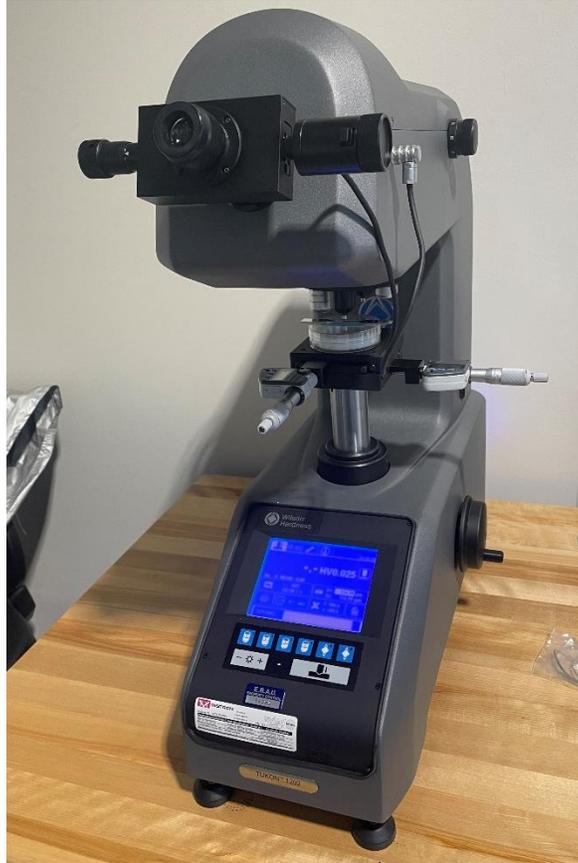
Figure A.5: Wilson Tukon 1202 Micro-Hardness Tester.
