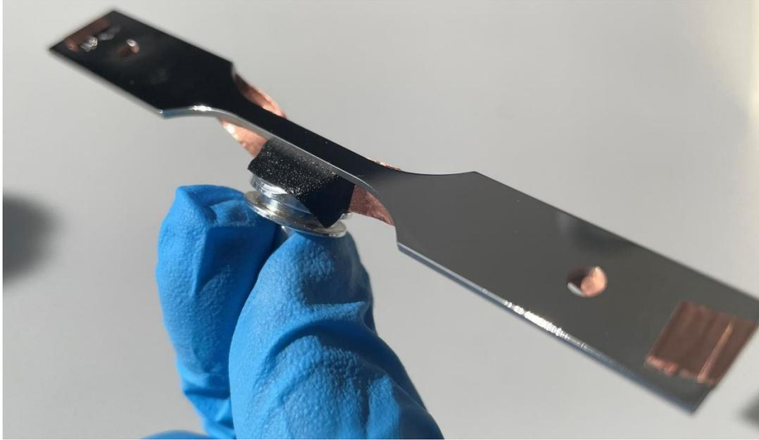
*Figure 3.5:* IN-718 sample mounted on 45° Aluminum holder with carbon and copper tape.
