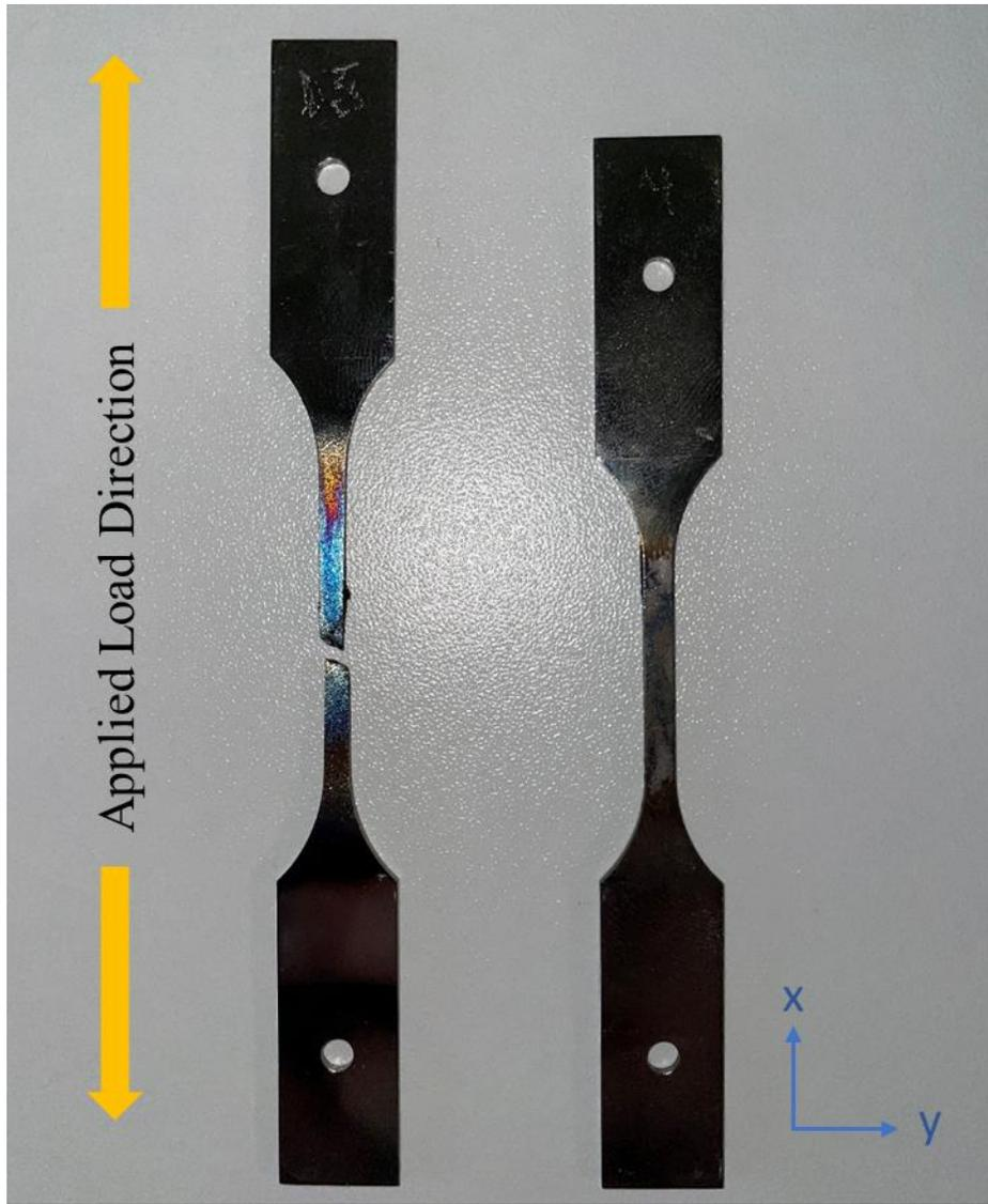
*Figure 4.1:* Fractured IN 718 Sample 1 next to Sample 2. Axis included for sample direction.
