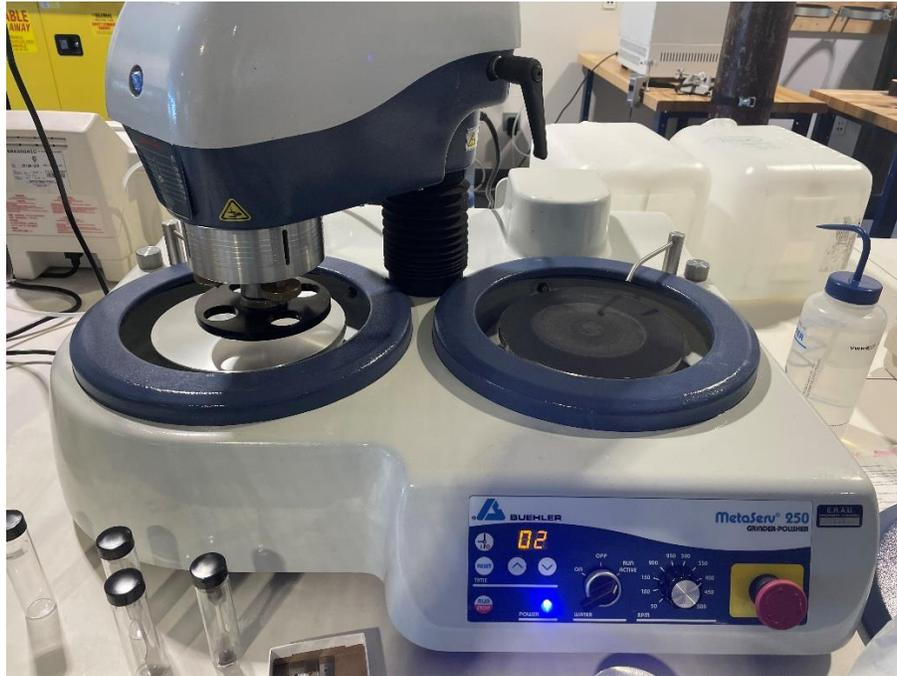
*Figure A.1: Buehler Metaserv 250 Semiautomatic Twin Polisher.*
