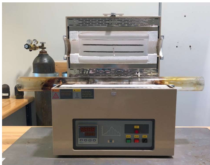
Figure 3.1 Tube furnace utilized in carbon fiber de-sizing.
