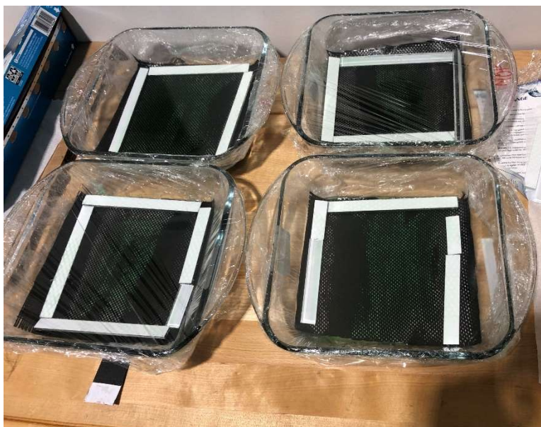
Figure 3.2 Carbon fibers fabrics submerged in MOFs growth solution
