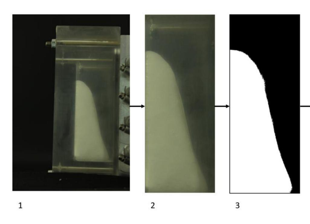
• When completed for all the collected images of a given melt, a melt fraction versus time graph will be created to study the phase change and create a benchmark to be used for potential future numerical simulations
