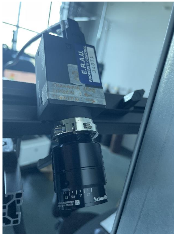
Figure 3.5 The DIC camera with attached lens
