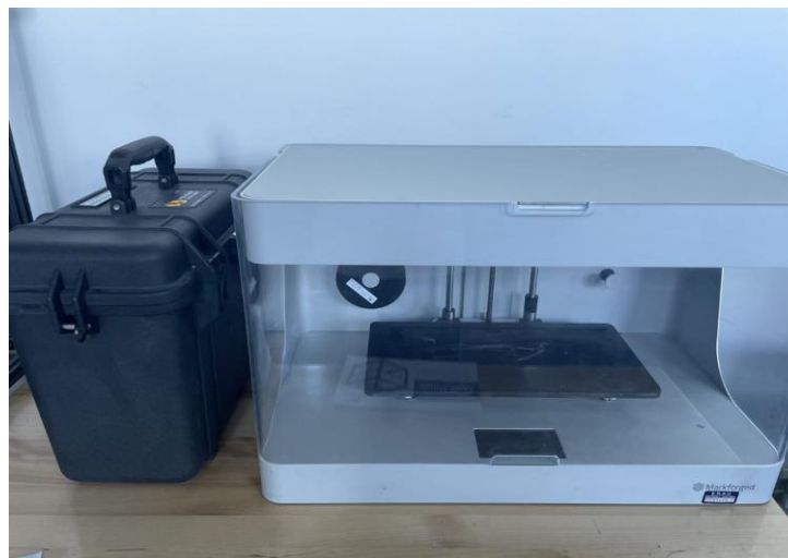
Figure 3.4 The Mark Two (right) beside the dry storage container (left)
