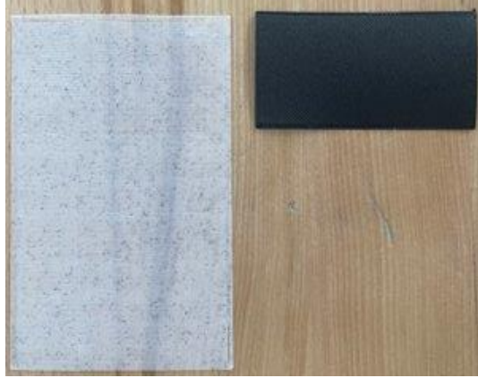
Figure 3.11 Comparison of the PLA (left) and the Onyx (right) prints
