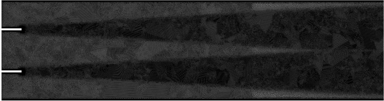
Figure 3.5 Wake refinement propagating off the splitter plate tips
