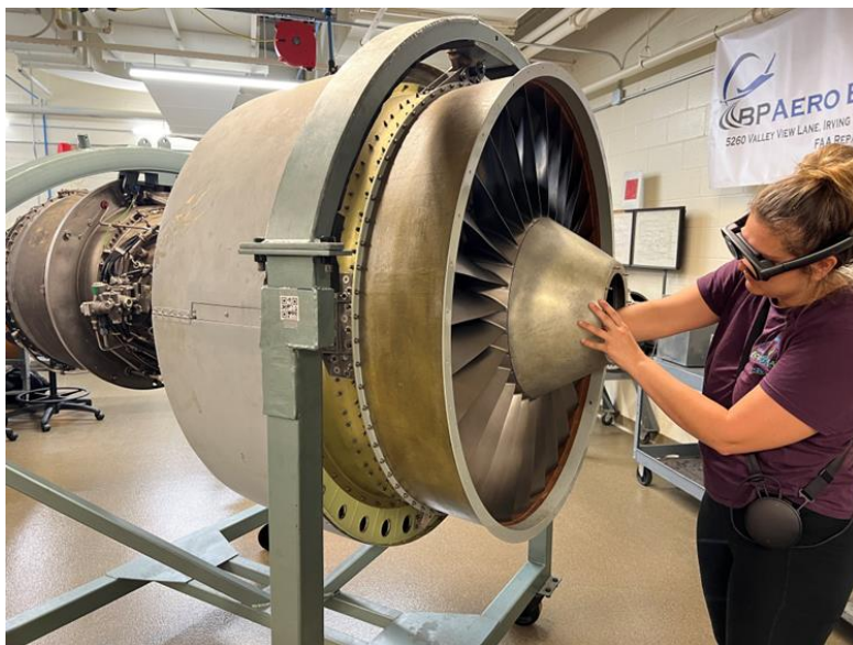
A User Wearing the Magic Leap 2 While Using the Fan Blade Replacement Application
