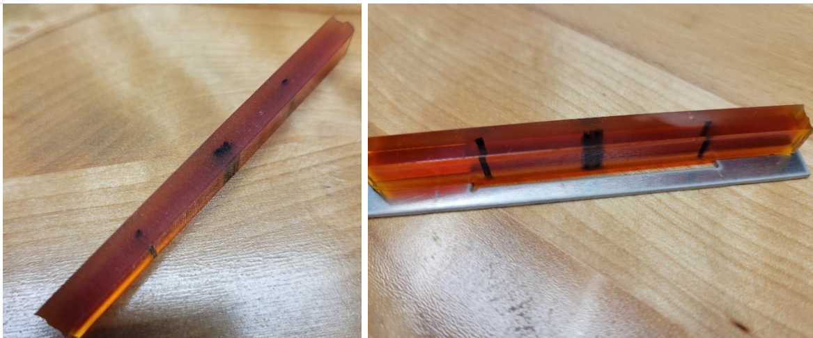
Figure 3.8 Initially cut sample (left), and sample after grinding and polishing (right)
