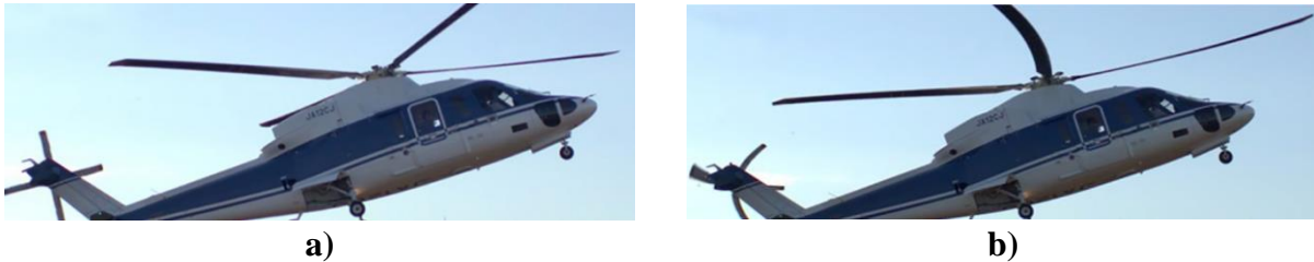
Figure 7: a) A picture of helicopter's propellers taken with a global shutter camera. b) The same photo taken with a rolling shutter (Paul, 2016).
