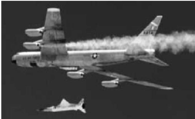
*Figure 2.14* The Pegasus rocket booster carrying the X-43A separates from NASA's B-52B [11].
