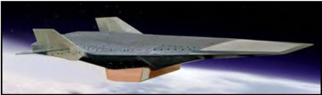
*Figure 2.12* The X-43A was a 12 foot long wedge-shaped hypersonic scramjet [4].
