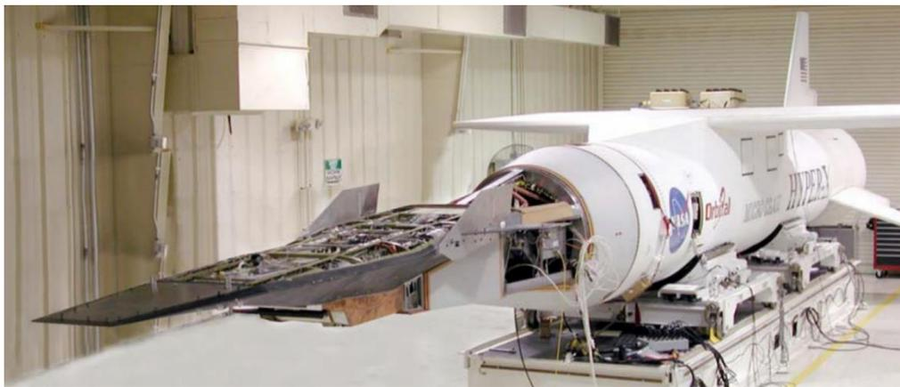
*Figure 2.13* A modified Pegasus rocket booster was used to accelerate the X-43A after separation from the B-52 [16].
