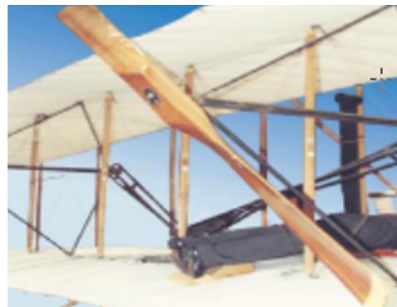
Fig. 2. Wright Brothers fixed pitch twin bladed propeller.
