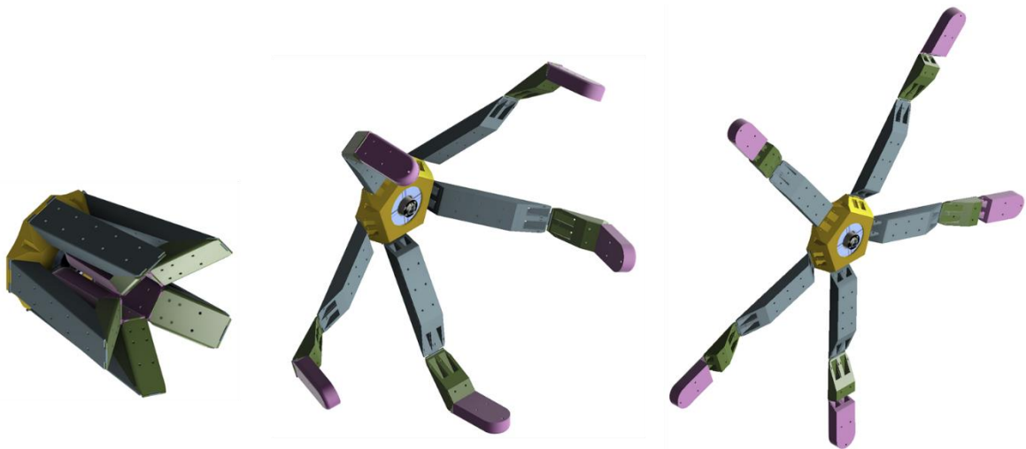
Figure 0.4 Images of Starfish moving from its compact to fully extended phase.
