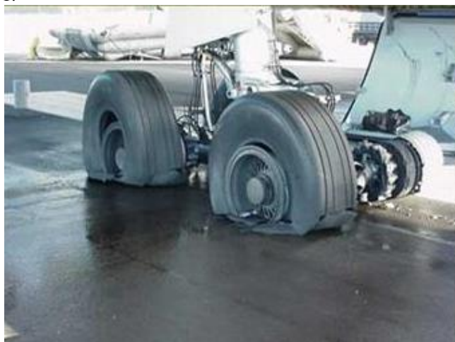
Figure 1, result of the hard landing.
