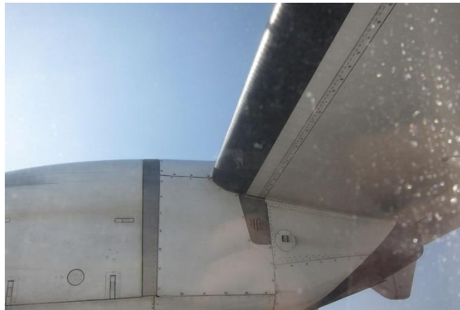
Figure 4, rubber leading edge for ice removal.
