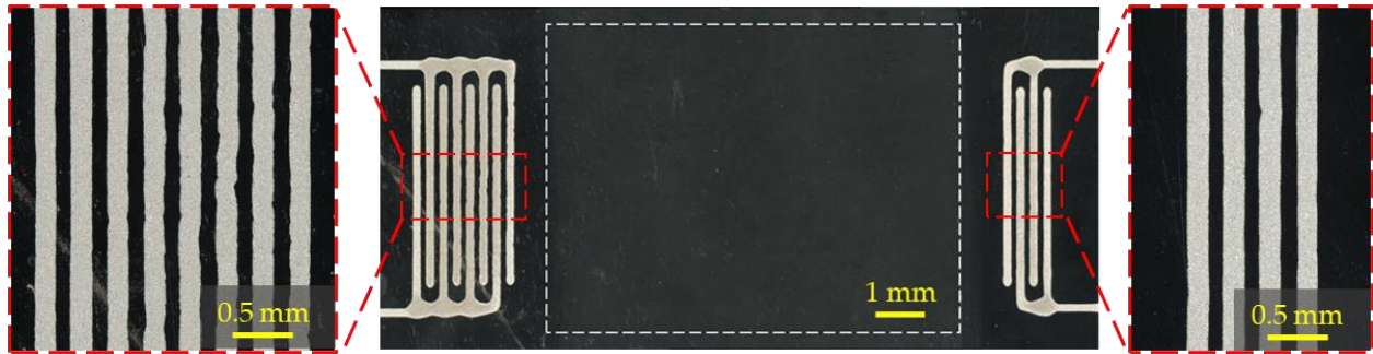
Figure 10.6 Microscope images of 3D printed input and output with ZnO sensing layer marked.
