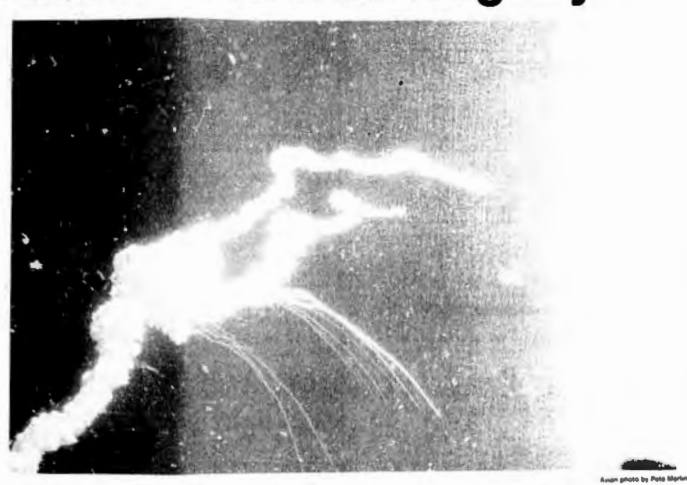
(Above) Aftermath of a disaster shows debris from the disintegrated Space Shuttle Challenger . The two solid rocket boosters continue to thrust, causing the twin corkscrew-like trails leading up to the right. (Sequence from bottom)
