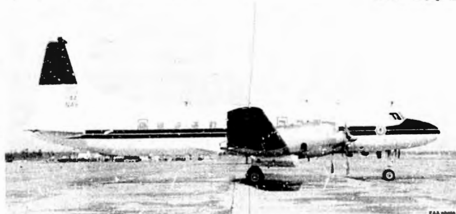
This Convair 580 with Allison twin turbo prop engines is flown out of the FAA Technical Facility in Atlantic City into local thunderstorms to collect lightning strike data on airborne aircraft.
