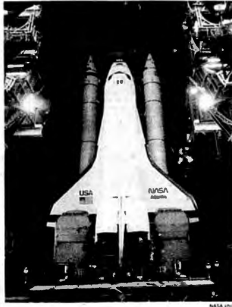
Atlantis will be rolled out to launch pad 39B next week. The spacecraft will undergo a series of tests including a simulated countdown and evaluation of a new weather protection system.
