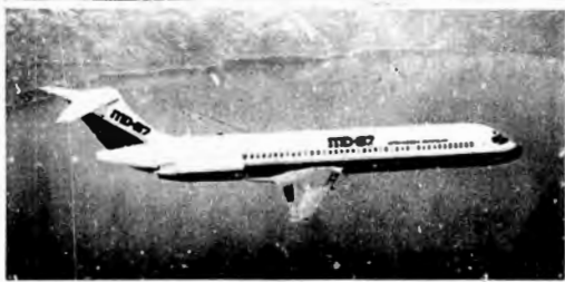
The MD-87 is a smaller version of the popular twins that maintain a high degree of commonality by using McDonnell Douglas MD-80 twin-jet that maintain the same cockpit, simulators and engine.
